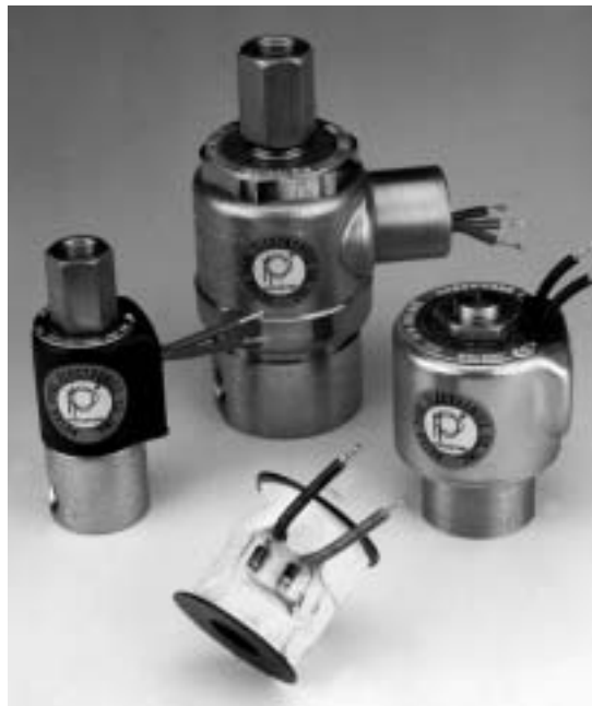
Location of the rectified fly back diode array in DC rectified solenoid valve coil is shown (cutaway). Most of our valves can be so configured, including the Models 50, 20, and 30 (left to right) above, all specified with diode rectified coils for the inherent low noise/low temperature provided by DC operation. They are used primarily for low noise/low temperature quiet locations such as hospitals and laboratories.
