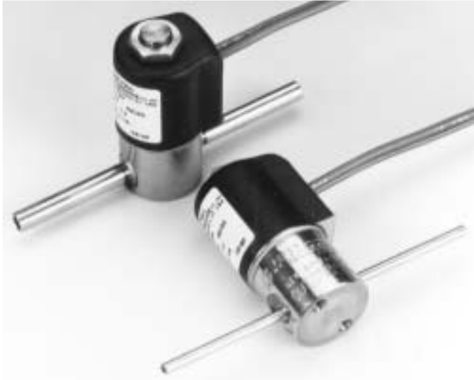
Two examples of the new, sealed, Peter Paul Series 50 solenoid valves for electronics and chip manufacture are shown. A 24 VDC, 7.0 watt, 1/16 orifice, 100 psi solenoid valve (top) is offered with grommet housing and 1/4" O.D. stainless steel tubing welded to the body; the sleeve assembly is threaded to the body and sealed with an elastomeric gasket. The valve below incorporates welded 1/8" O.D. input/output tubing but with body and sleeve assembly welded together, eliminating the gasket and threads, for total, positive, permanent sealing.
