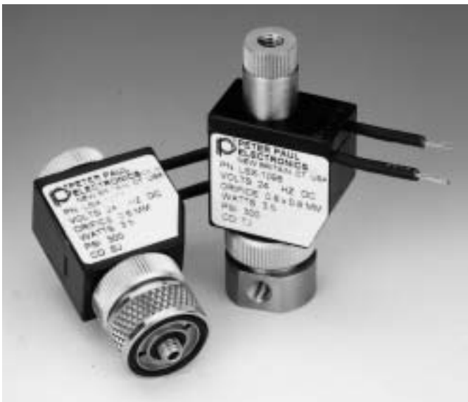
Two Peter Paul Series 58 valves with stainless steel bodies are (left) 2-Way, NC, stud mount, and coil with lead wires; (right) 3-Way, NC, piped exhaust, 10/32 ports, and coil with lead wires.
