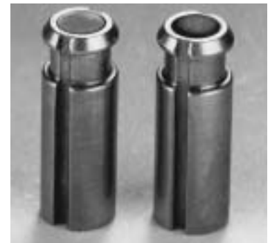
Solenoid valve plunger travel stroke is typically 0.020 to 0.050 in., depending on orifice size. Choosing the wrong seal material could literally shut off the valve flow. Notice the swelling in the seal at right.
