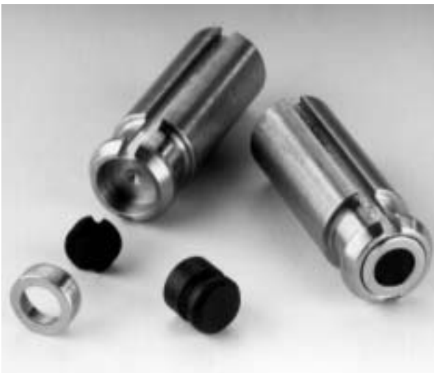
We have developed a new and significant cost saving procedure for laser cutting Kalrez® seals from sheet stock for solenoid valve plunger assemblies. Previously (and difficultly) molded seals requiring more than double the amount of Kalrez have now been replaced by a Kalrez seal disc and stainless steel seal cup which are press fit into the plunger. Shown here, clockwise from left, are the new seal cup, seal, and plunger; a Series 52 solenoid valve plunger assembly complete; and a typical molded Kalrez seal from a previous solenoid valve design.
